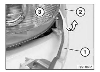
Carefully feed out trim (1) at front side section (2) in direction of arrow.
