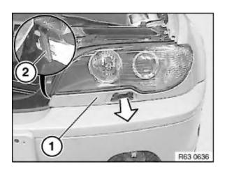
Unclip trim (1) at point (2) and feed forward out of lower catches.
