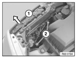
Release screws (1) and (2) and lever out headlight towards front.
