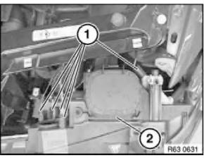
Unlock plug connections (1) and disconnect. Remove headlamp (2).
